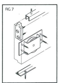
5. Cut 60-2 aluminium bottom track to length. Track can be recessed into bottom timber or sit proud on top. Fix with no. 3 x ½" long woodscrews — fig 4.
