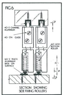
3. Cut out recess in top corner of door to take a 40-374 nylon guide. Repeat other end but do not screw in guides — fig 2.
