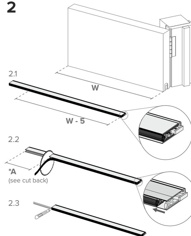
**2.1** Measuring from the actuator end of the product, mark with a pencil the width of the door less 5mm (W-5).
