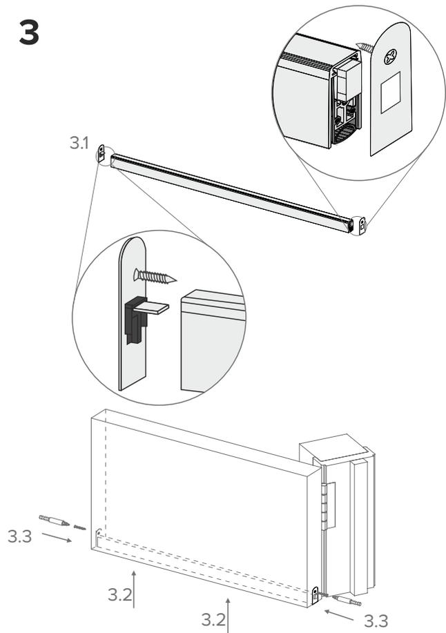
**3.1** Ensure the black plastic distance piece is in place on the end plate.
