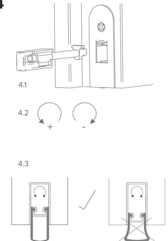
**4.1** To adjust the seal remove the actuator.
