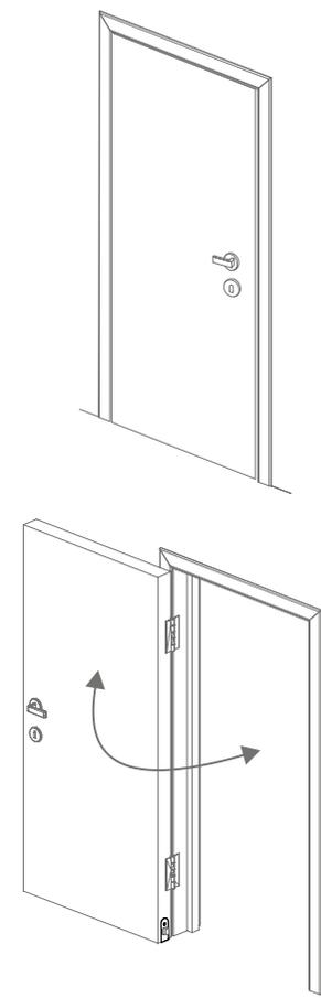
**5** Open and close door to test seal drop.
