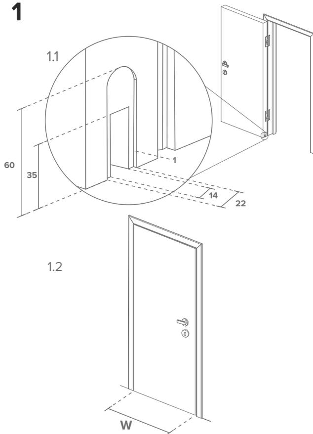
**1.1** If installed, remove door from hinges lay on its side and restrain firmly. Using a router machine mortise a 35 x 14mm groove the full width of the bottom of the door as per diagram. Machine mortise the end of the door for end cap as per diagram 1.1 with a depth of 1mm each side.
