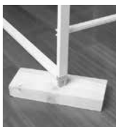
Wood block to protect the floor
